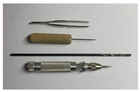
They consist of a common household tweezers, a .036" diameter drill bit mounted in a dowel to provide additional torque (yes, a tool specifically used to unclog Autopoint pencils that utilize "real thin" leads -thank you Father Terry RIP), a 1/8" diameter drill bit with an extra-long shank, and a medium pin vise with a pointed tip on the pin.
